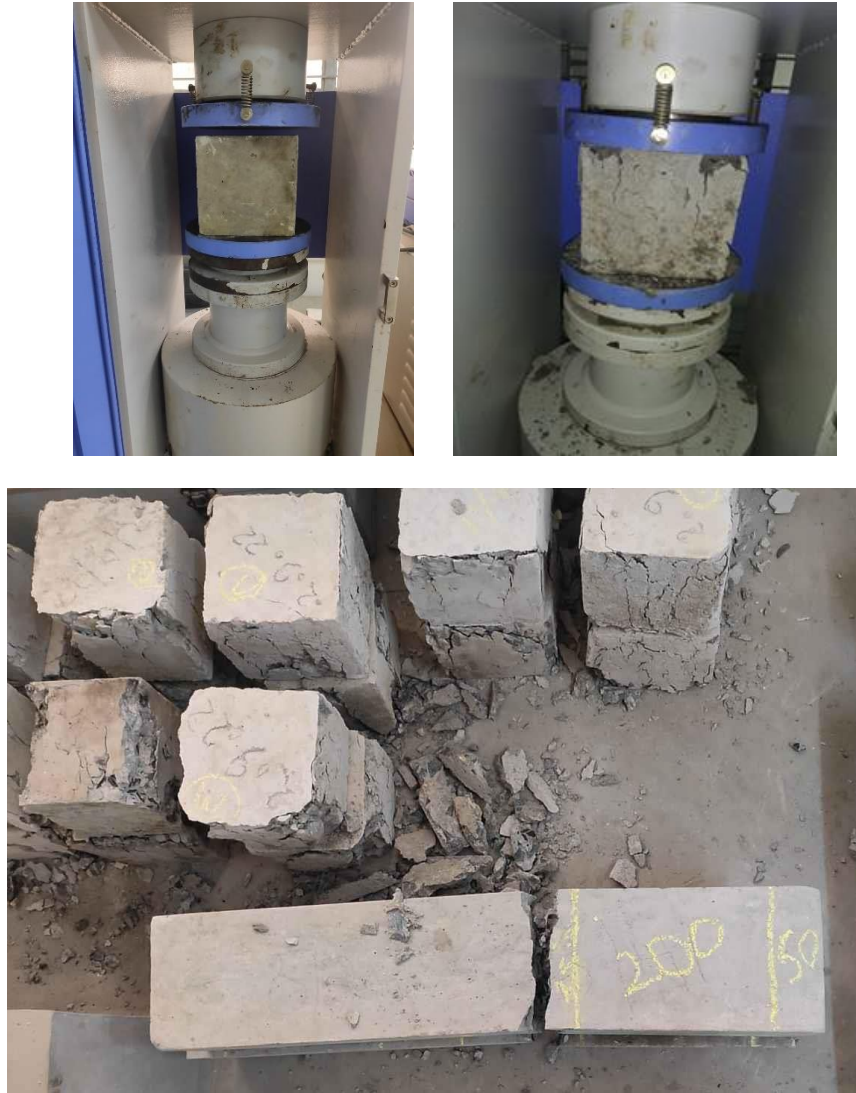
Figure 3 – Lab Performance for Strength Test of Coconut Shell Concrete
